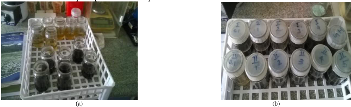
Fig. 3. Samples Containing Activated Carbon with different Dosages (a) Before addition Activated carbon (b) After addition of Activated Carbon
