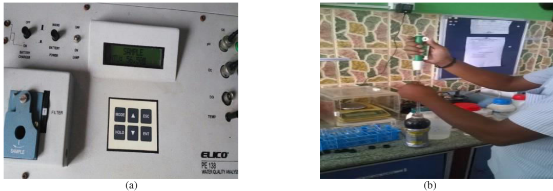
Fig. 2 Testing of Samples for Physical and Chemical Parameters (a) Check for Turbidity value (b) Collection of Sample for COD
