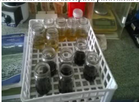
(a) (b) Fig. 3. Samples Containing Activated Carbon with different Dosages (a) Before addition Activated carbon (b) After addition of Activated Carbon
