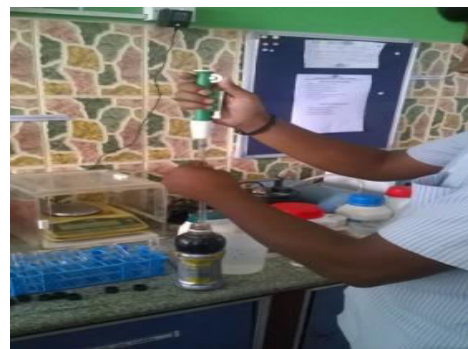
(a) (b) Fig. 2 Testing of Samples for Physical and Chemical Parameters (a) Check for Turbidity value (b) Collection of Sample for COD
