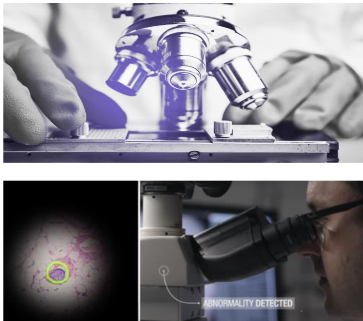
Figure 1: During observation, the AR microscope can overlay a digital image of a biological material with an outline.
