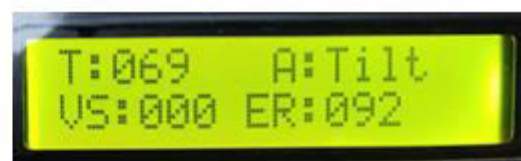
Fig 10: MEMS sensor at tilt position and High engine emperature detected
