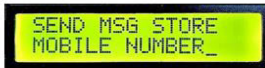
Fig 6: LCD Prompt: Send Message to GSM Module SIM Number for Number
