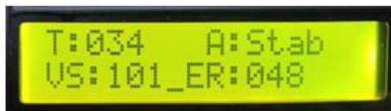
Fig 11: Vehicle Speed exceeding 100kmph
