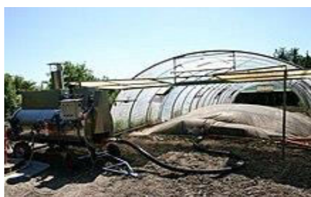
Sheet steaming with a MSD/moeschle steam boiler (left side)
