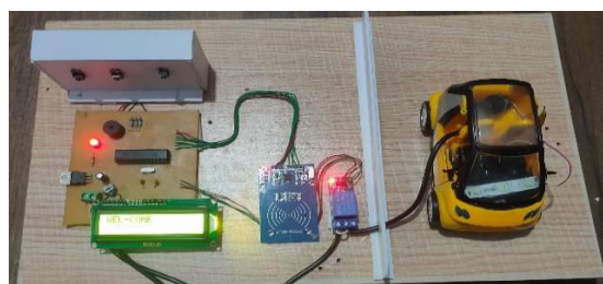
Fig 2: System prototype of RFID based EV charging station.
